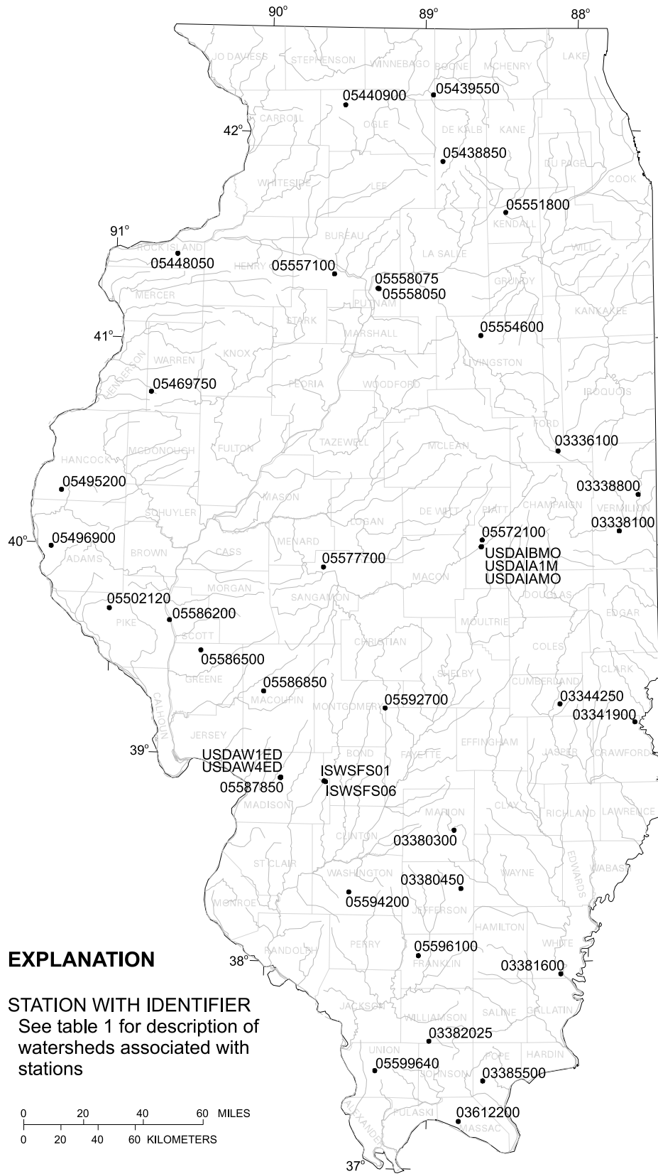
Figure 1. Location of stations where rainfall and discharge data were collected and used in the development and verification of equations for estimating time of concentration and storage coefficient for the Clark unit hydrograph for small watersheds in Illinois.
